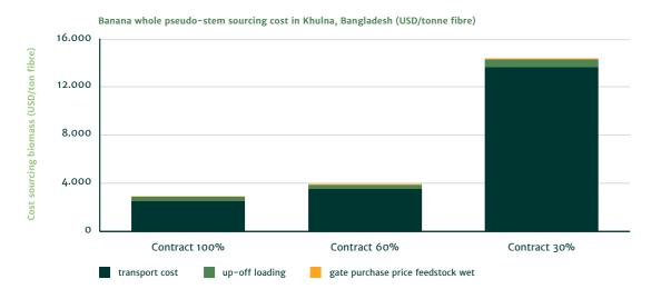
vesting of the whole pseudo-stem up to the roadside is assumed to be less labour intensive than the first scenario, but the volume transported is bulkier. Transportation costs are therefore higher per tonne fibre and more residues are removed from the field, which would need to be transported back to the field after extraction of the fibres at the plant.
