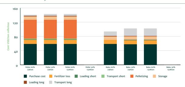
Figure A5.5: Distribution of cost over cost items for sugarcane trash pellets and bales at different sourcing levels for Indonesia
