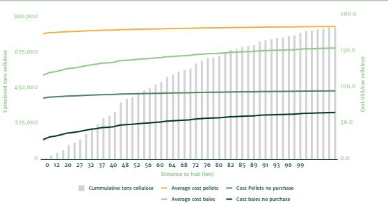
**Figure A5.7:** Biomass delivery cost at different biomass chain options combining trash and bagasse to a medium size cellulose dissolving plant in Uttar Pradesh (India)
