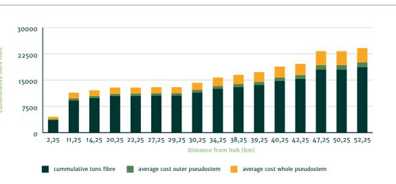
Figure 4.8: Comparison between delivery cost of outer and whole banana pseudo-stems, and distance to fibre extraction plant in Samut Prakan, Thailand
