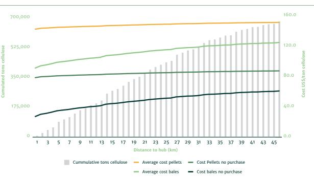
If the purchase costs are not considered, it can be concluded that the lowest at-gate cost for rice straw delivery at the dissolving plant gate is found in the two hub locations in Indonesia where bales can be delivered to a medium and large dissolving plant at 28 and 35 USD/ton cellulose, respectively.
